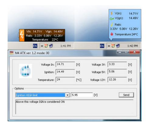
When you connect M4-ATX by USB with your PC, then you can control voltages and temperatures with the control software. With the Advanced software version you even are able to change the behavior of the power supply.
