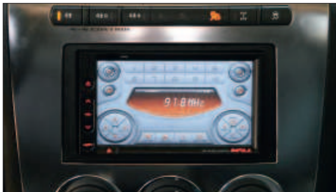
▲ The Infill G4 requires a Double DIN space in your car's dashboard, which means it takes up twice the space of a regular automotive hi-fi head unit.
