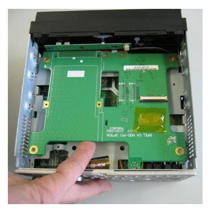
To remove the board completely, the cable has to be plugged off:
