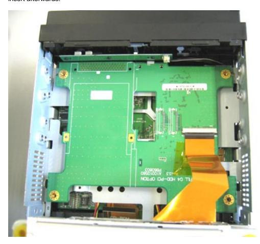
Now the ribbon cable gets connected to the DVD drive, the board gets screwed tight and the cover of the enclosure gets put-on and the barebone gets screwed on:
