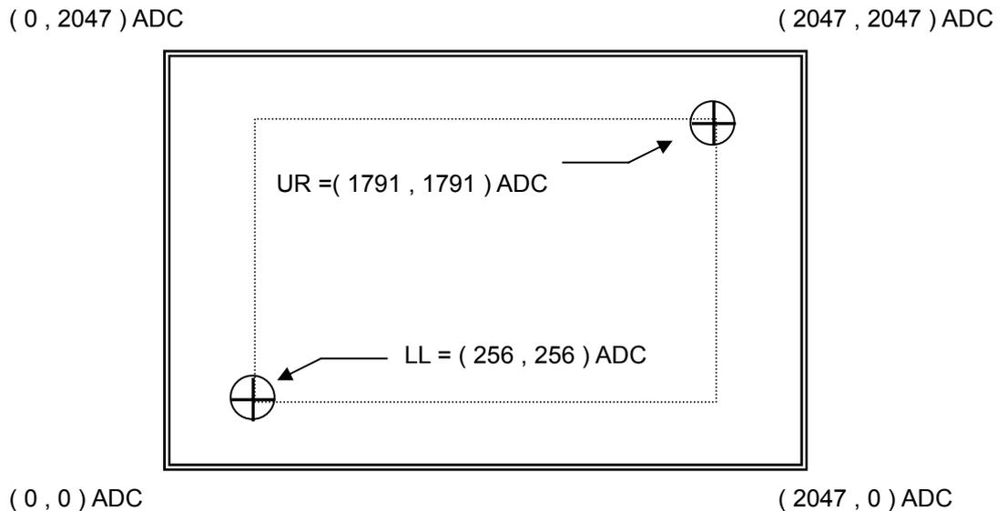
1. LL and UR are the calibration points of touch panel, the points are setup at
