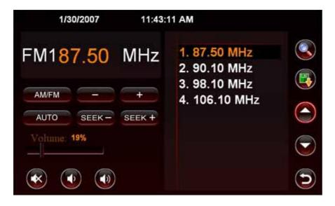
Manufacturer of the 7" display panel is Sharp, therefore it sires very high quality. The physical resolution is 800x480 pixels, while the luminance density amounts to 400nits. The touch screen registers input very quick and also works well when you use your finger to operate it. Unfortunately, the surface of the display reflects but other displays are reflecting as well. It could become difficult to read with direct sunlight.
