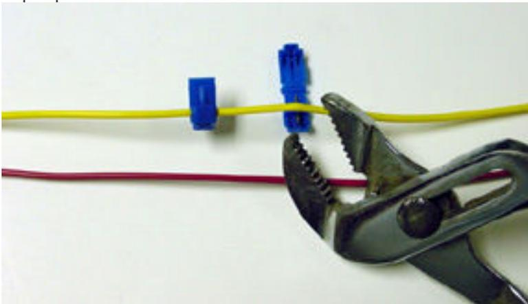
9. Now you can attach male terminal to an appropriate T-Tap according to the harness diagram and color of the adapter wire
