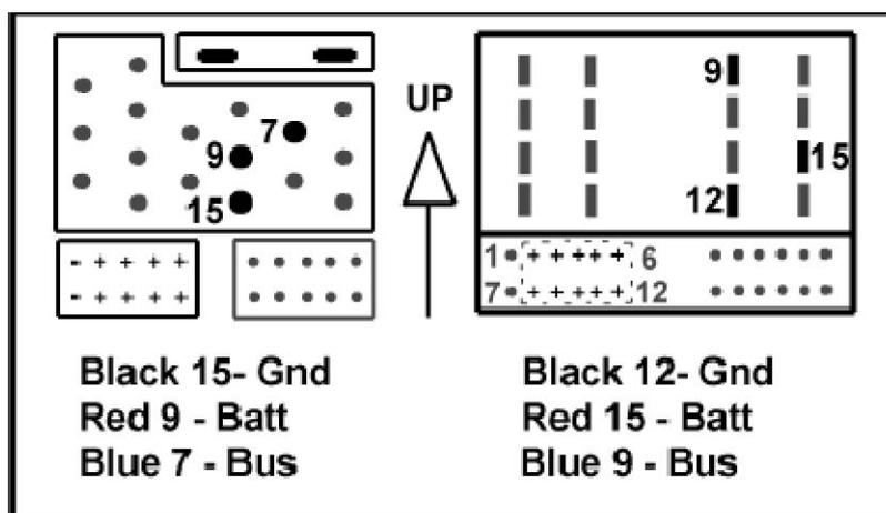
4. 3 wires coming out of adapter are marked with the colors. Depending on your harness you need to connect adapter wires to the appropriate car stereo wires according to the picture above
