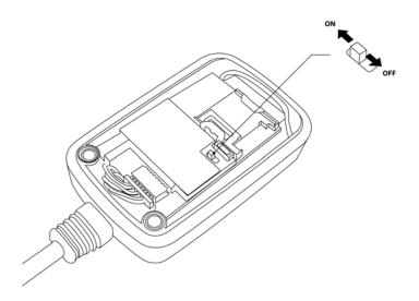
After connecting the power, please open the back cover and adjust the power switch to ON position.
