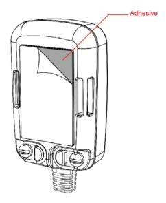
You could tear down the cover of double side tape and stick GTR-129 to the installation position.
