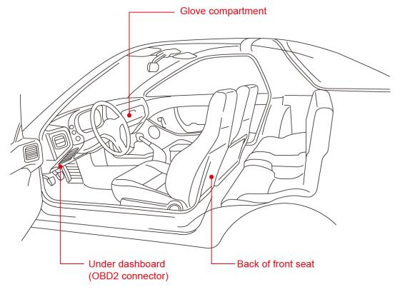
If you'd like to install GTR-128/GTR-129 at the OBDII connector of vehicles, please connect GTR-128/GTR-129 with the OBDII power cable firstly, then you could connect the OBDII power cable to the OBDII connector of vehicle as the picture below.
