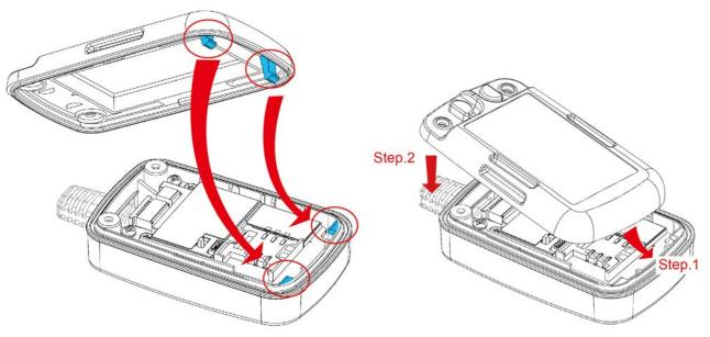
Step 1: Please align the latches of the back cover to the indentation of the device.
