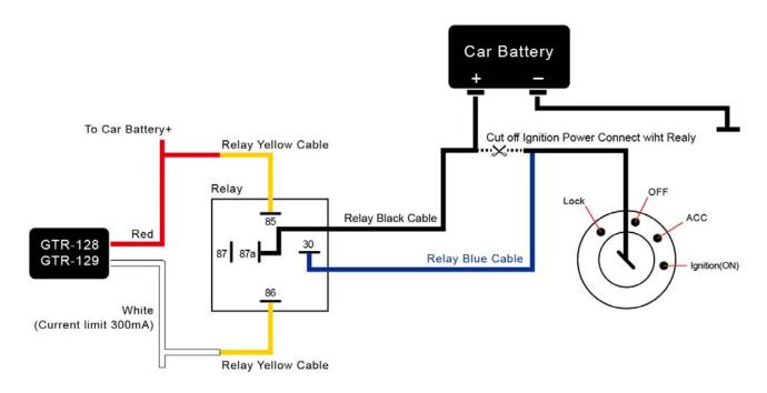
Connect the white wire from GTR-128/GTR-129's cable to the yellow wire of relay. For the other connections, please refer to the diagram above.
