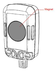
You could install the GTR-128 to a metal surface. The magnet on the device would attract the metal surface.
