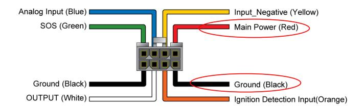
Connect the red wire from the cable to a power source of 9~36 V. Connect the black wire to ground.
