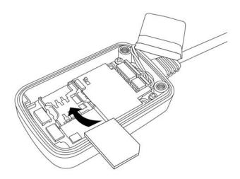
Unscrew the cover of device. Insert SIM card with the copper contacts face-down and the notch on the SIM card at the right side of the SIM slot.
