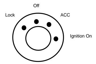
Connect the orange wire from the cable to ACC position of vehicle. Connect the black wire to ground.
