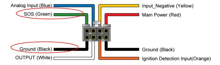
One end of the button must be connected to the SOS line and the other end must be connected to the ground line.
