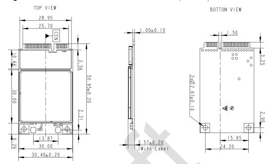
Figure 6-1 Dimensions of the ME909s Mini PCIe module (Unit: mm)
