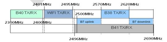
The two systems interfere with each other because of nonl inear characteristic of LTE Band 38/40/41 and Wi-Fi transmitter. The main impacts are as follows:
