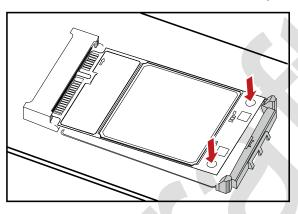
Step 3 Use a screwdriver to fix the Mini PCIe Adapter on the main board with two screws provided in the Mini PCIe Adapter packing box.
