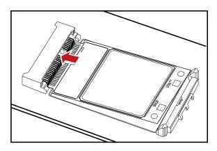
Step 2 Press downwards to fix the Mini PCle Adapter in the module slot.
