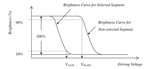
$Vop = (V_{10,ON} + V_{90,OFF})/2$
