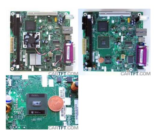
All in all one DDR2 RAM can be installed onto the motherboard only. The 2 SATA ports, one IDE cable and the cable connector are placed at the outside of the motherboard. In contrast with to the older GLY series, you now have the possibility to use the complete picoPSU series, for example to install the picoPSU120WI, which is a little thicker.
