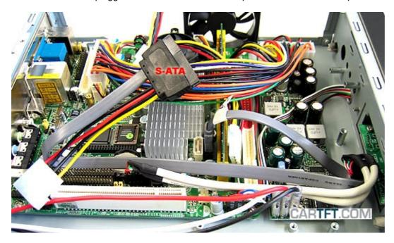
Then you connect the S-ATA cable with the HDD and also both Molex connection plugs together.
