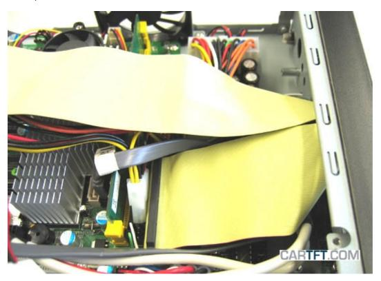
The IDE cable gets pulled through the framework opening.
