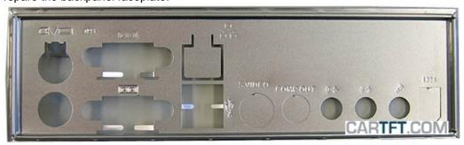
Then you insert the backpanel faceplate into the case and afterwards you insert the motherboard. When installing the motherboard, you have to look, that the motherboard is pressed at the backpanel, so that the sockets are reachable.
