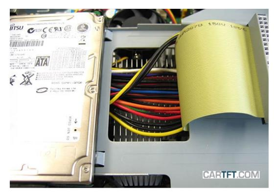
The disk drive blank faceplate is then screwed onto the case again. The cables must therefore be laid so, that no cable is squeezed. The 3 connection cables of the m2 ATX (duration plus, igniting plus, mass) are led behind out of the case there where the already removed power connection was..
