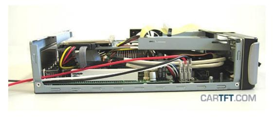
For lack of space there is no need for so much IDE cable length, so the IDE cable gets cut after the IDE plug:
