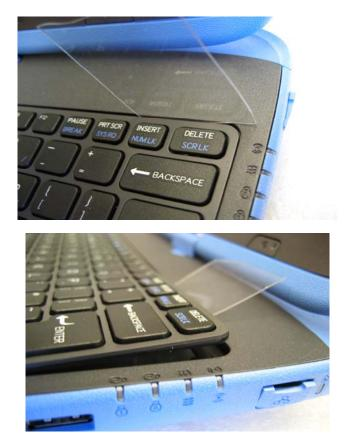
Insert the first card on height of the "Insert"-Button between casing and keyboard.
