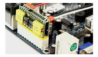
2) Connect a 6-26VDC power adapter (or any 6-26VDC source) to the input connector.
